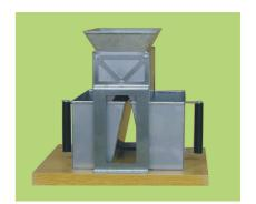
A manual sample divider is used to accurately divide a sample of cereals, pulses, oilcake or similar products into smaller samples of equal size or into one sample of a reduced size as requested.
